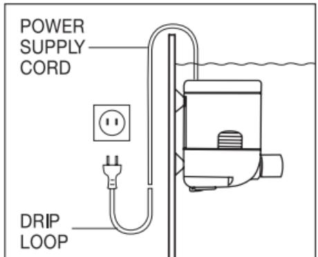
The “drip loop” is that part of the cord below the level of the receptacle, to prevent water travelling along the cord and coming in contact with the receptacle.
